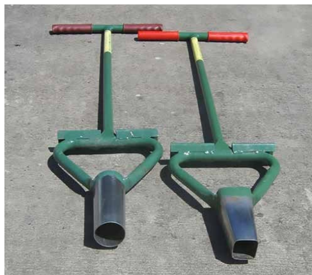
Figure 7: Hamilton tree planters with round or square ends for different shaped seedling tubes. Photo: AMLR NRM Board.
