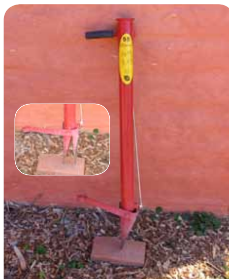
Figure 15.7: A Potti-Putki tree planter. Inset: planter with beak open. Photos: D. Carr
