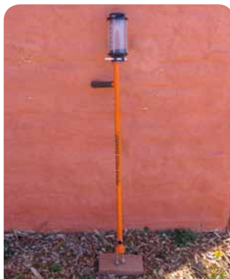
Figure 15.9: This niche seeder moves away a small amount of soil then drops a specified amount of seed from the bottle on the tube. Photo: D. Carr
