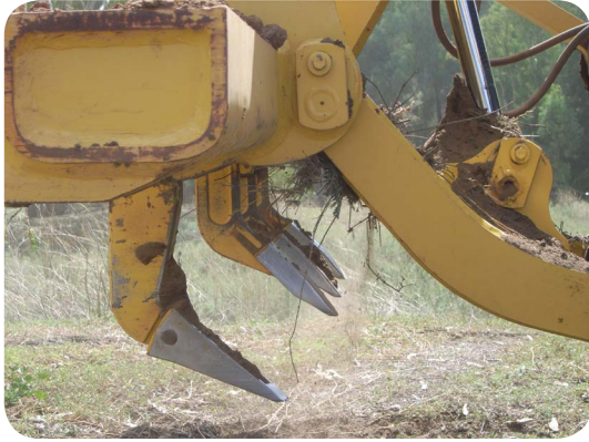
The ideal implement for deep soil cultivation—a three tine scarifier with deep ripper chaser.
