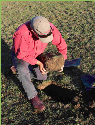
Step 1: Get a cube of soil approximately 20cm each side
