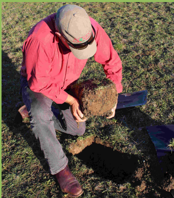
Step 1: Get a cube of soil approximately 20cm each side
